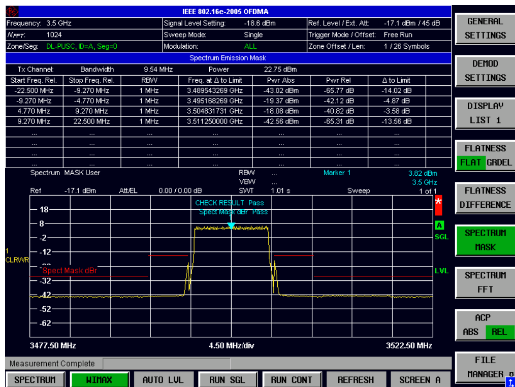
Fig. 54 Spectrum Emission Mask Results
