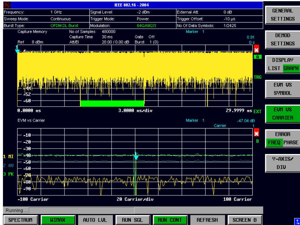
Fig. 24 EVM vs Carrier Results (SISO-OFDM)
