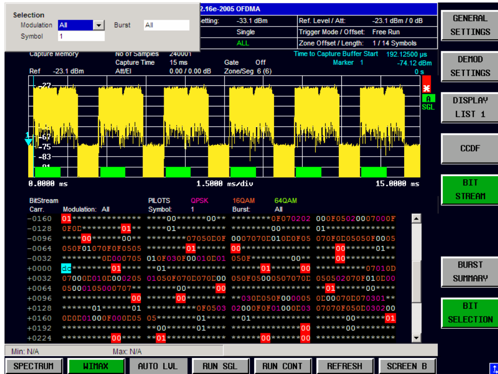
Fig. 50 Bit-Stream for OFDMA, showing the Bit Selection dialog and highlighted erroneous pilots.
