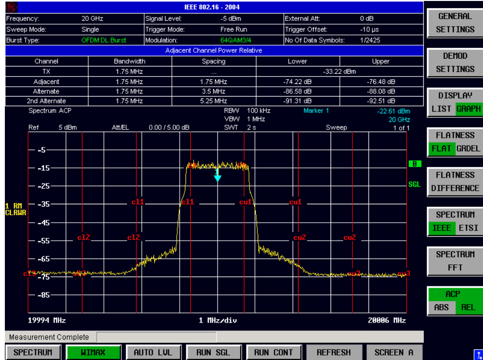
Fig. 59 Spectrum ACPR Results (example)
