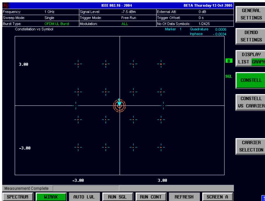
Fig. 115 IQ imbalance influence on the unallocated carriers using subchannel index 4
