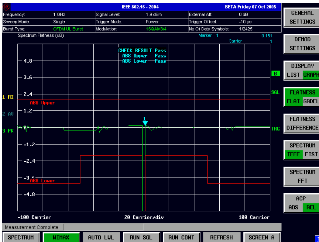
Fig. 114 Spectrum flatness using subchannel index 4
